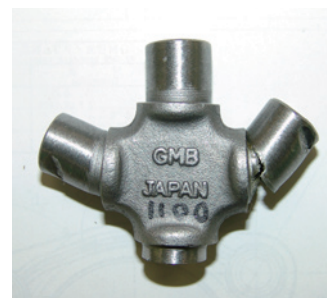
Picture of Imitation GU-1100, which was transformed and destroyed by only 65.6kN.
