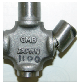
Instances of transforming / collapsing easily because breaking strength is extremely low
