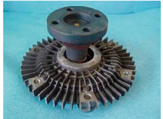
Fan clutch bearing blocked ➔ breakage
